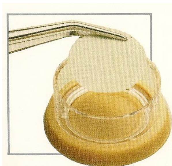
Removal of the Anopore membrane from the Anocell device
