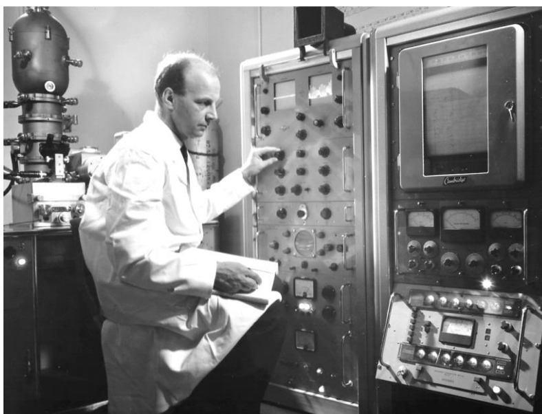
Henry Lamb operating the early Electron Probe Microanalyser
