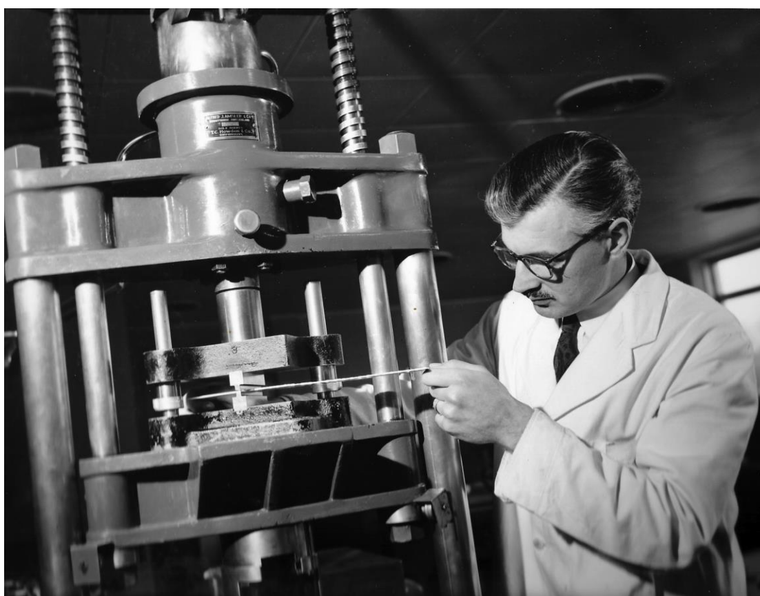
Plane Strain Compression (PSC) Testing in the mid-1950s
