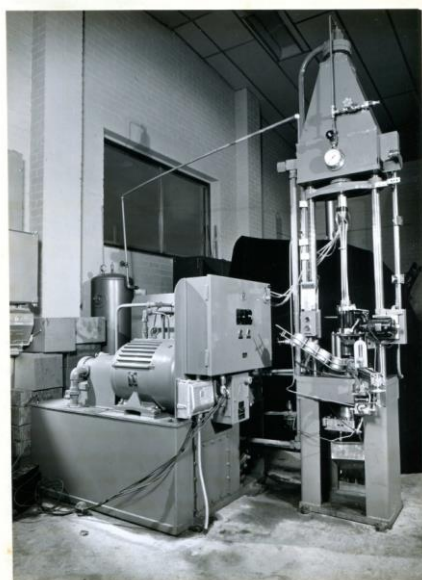
Figure 5. Hydraulic press, showing (right) the press and tools and (left) the power unit and oil storage tank.
