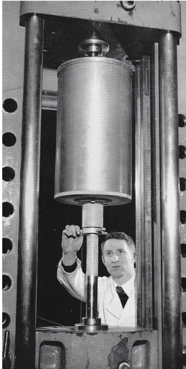
Ray Durham undertaking a low temperature tensile test
